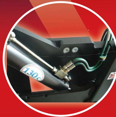
130 degrees rotation using a single hydraulic cylinder
